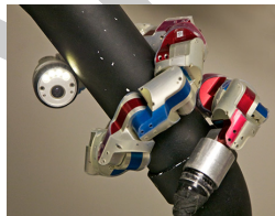
modular snake robot (Carnegie Mellon)
